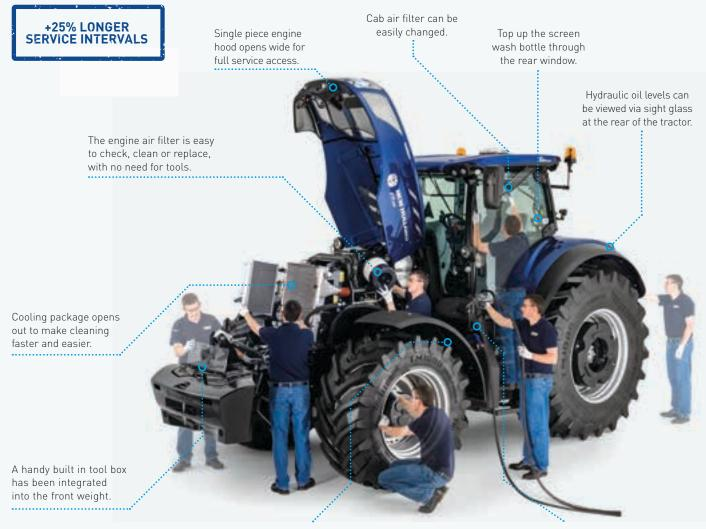
Engine oil check and fill points are easy to reach, with no need to lift the hood. This makes routine checks faster and servicing simpler. The best-in-class 630 litre fuel tank (T7.290 and T7.315, optional on 270) means you can work the whole day long and well into the night without the need to refuel. True 24 hour productivity courtesy of the T7 Heavy Duty range.
